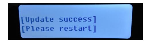
You can verify that the Firmware has been updated by exiting the Firmware Update Utility and with the Printer back in REDAY state, go to the GENERAL tab of the Printer Driver, selecting the Preferences button, select the Maintenance tab, Printer Settings button to select the VERSION INFO under the Parameter Items to then view the various Firmware levels, as outlined in steps 3,4 and 5 above.
