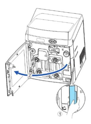
2) Push the Ribbon Lock ① clockwise to unlock the ribbon cartridge and pull out the whole cartridge ②.
