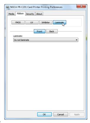
③ Laminating the back side, select "Laminate" button and the "Back" button. Change the option to "Laminate back side".
